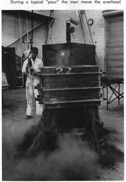
HOT SAND of the mold drops away as outside steel "flask" is pulled away by Donald Quayle. He controls crane with pushbutton.
